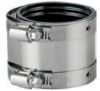
Connects no-hub drain pipes of dissimilar materials. Can be used on any combination of plastic, steel or extra-heavy cast iron pipes. Series 300 stainless steel shield and neoprene gasket. Not recommended for use underground.
