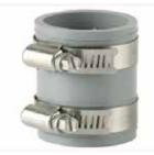
Standard: Ideal for extending, altering or reparing drain pipes. Can be used for installation of condensate lines on air conditioners. Not for use in potable water applications Tubular: Quick and easy way to extend, alter or repair any combination of 1-1/2" or 1-1/4" brass or plastic drain pipes. For above ground use only. Made of flexible PVC.
